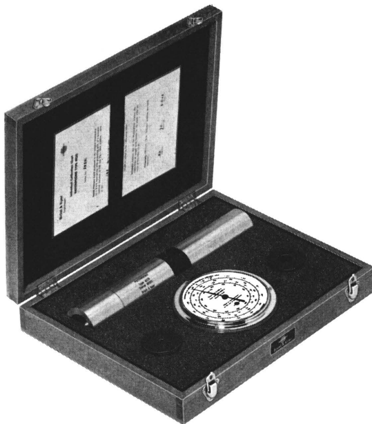
Fig. A.3. Pistonphone Type 4220 in case with Barometer and Coupling Adaptors for fitting to the different B & K microphones.
